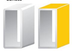
Aluminum box sections are extruded, heat cured, with high torsional stiffness. Cross-sections: 22-23/50 and 25/60mm Wall thickness: 1.5 to 2.3mm, depending on type and length
