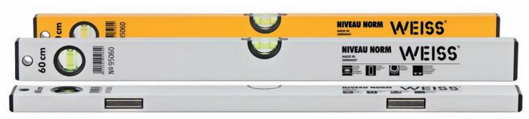
Strong aluminum box section, 22/50mm, sharp-edged, extruded, heat cured, with high torsional stiffness, and usable as a drawing aid on all sides.
