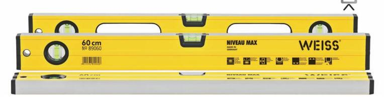
The extremely strong aluminum box section is 25/60mm, extruded, heat cured, with thick walls and reinforcing ribs for high torsional stiffness - the alternative to the die-cast spirit level. Usable as a drawing aid on all sides.
